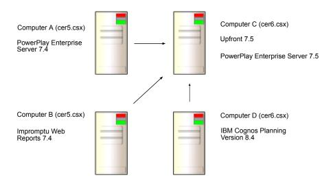
To configure this environment, you use both Configuration Manager 7.4 and Configuration Manager 7.5. You can complete the required configuration separately on each computer, or you can manage the server configuration files to import configuration information between computers.
